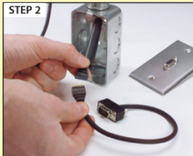
STEP 2 Slip shrinkable tubing onto cable, mate the breakaway connector matching alignment arrows and secure.
